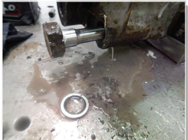
Ph (8) - Gear Housing - Reference - Water Contamination
