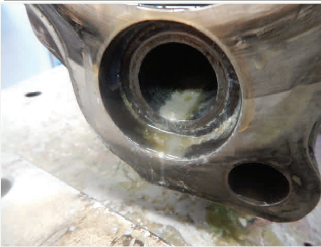
Ph (7) - LP Accumulator - Reference - Damaged diaphragm.
