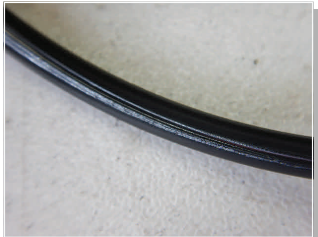
Ph (14) - Damping Seal Energiser - Reference - Over heated / Compression Set
