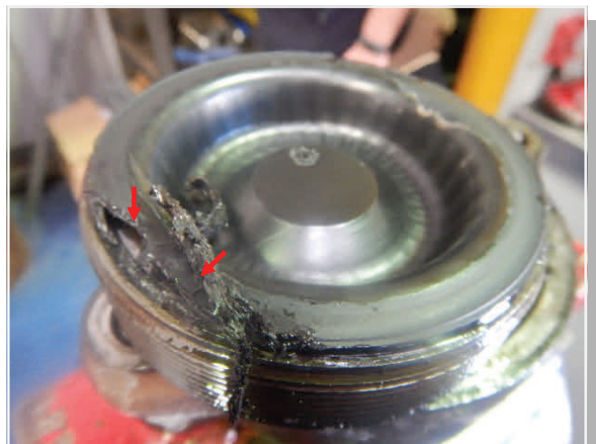
Ph (4) - Cover Plate - Reference - Cracked on bottom strapping bolt mating face (require weld and machine).
