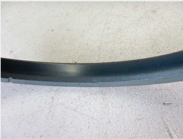
Ph (13) - Damping Piston - Reference - Evidence of over feeding. Damping piston to shoulder contact
