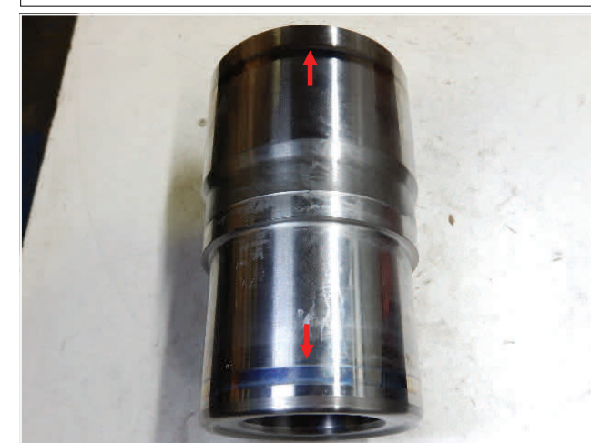
Ph (10) - Damping Housing - Reference - Evidence of over feeding. Damping piston to shoulder contact
