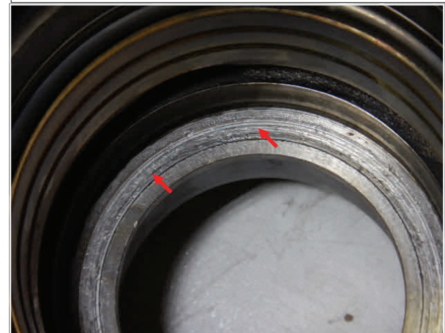
Ph (10) - Damping Housing - Reference - Evidence of over feeding. Damping piston to shoulder contact
