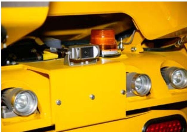
The MT6020 is standard equipped with a rear vision camera. A small detail, but definitely worth viewing - is the standard equipped camera for improved operator's visibility.
