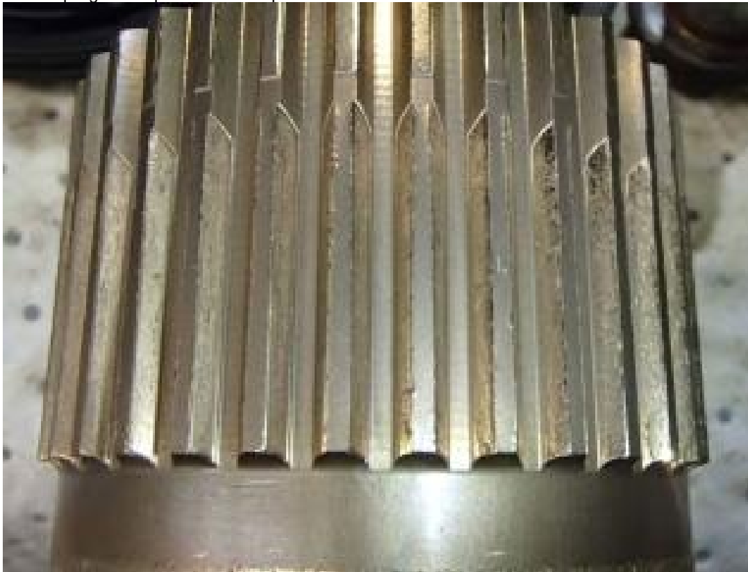
1 The coupling outer splines are worn past service limit.
