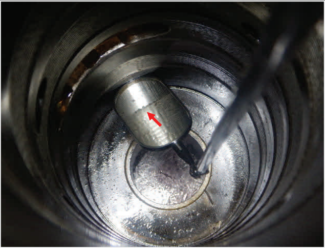
Ph (15) - Impact Body - Reference - Cavitation on top of rear land of cylinder bore.
