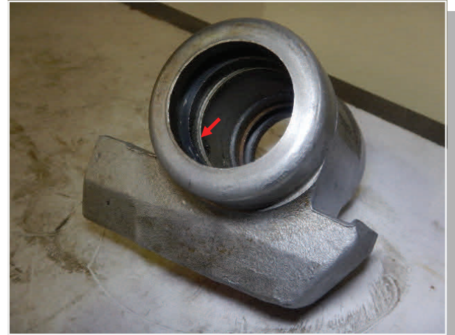
Ph (10) - Seal Housing - Replaced - Seal grooves corroded and damaged.
